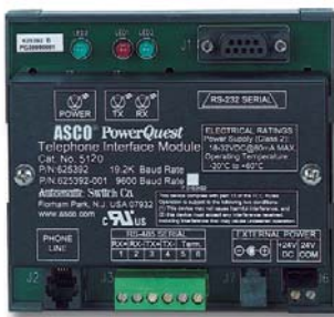
Fig. 19: Telephone Interface Module
